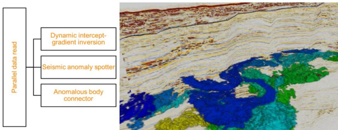
**Figure 1** A framework to preliminarily screen large seismic volumes for AVA anomalies (left). Each component runs in parallel on a Linux cluster environment and can be used to extract geobodies (right).
