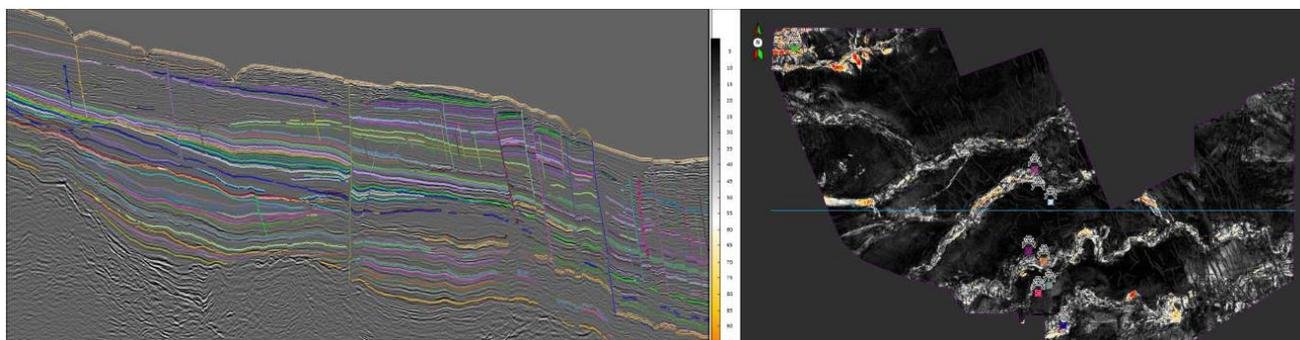
**Figure 2** A seismically derived geological model was created from the 3D seismic and used to visualise depositional geomorphologies.
