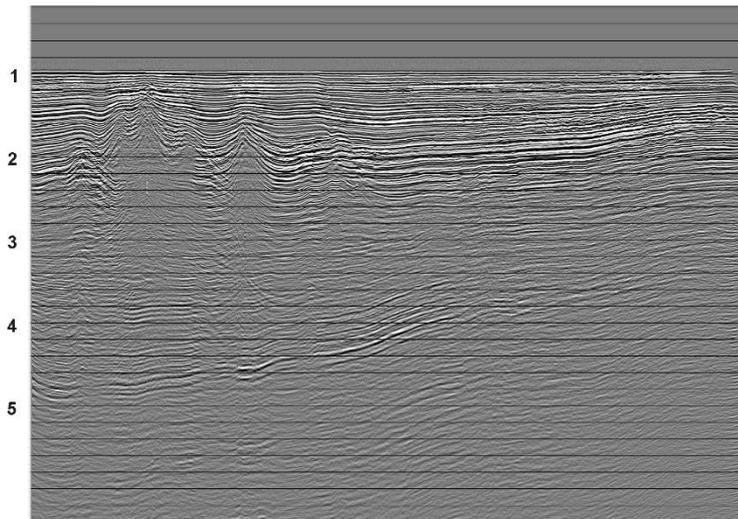
Figure 3. New SEGMENT project migrated profile – Lake Malawi. Image from Central Basin showing pre-rift basement reflections and mud diapirs. Processing by T. McCartney, Syr. Univ. doctoral candidate.
